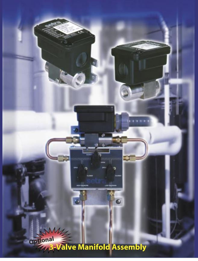
Setra Systems Model 230 is a high output, low differential pressure transducer designed for wet to wet differential pressure measurements of liquids or gases. A fast-response capacitance sensor and signal conditioned electronic circuitry provide a highly accurate, linear analog output proportional to pressure. Both unidirectional and bidirectional pressure ranges are available for applications with line pressure up to 250 psig.
